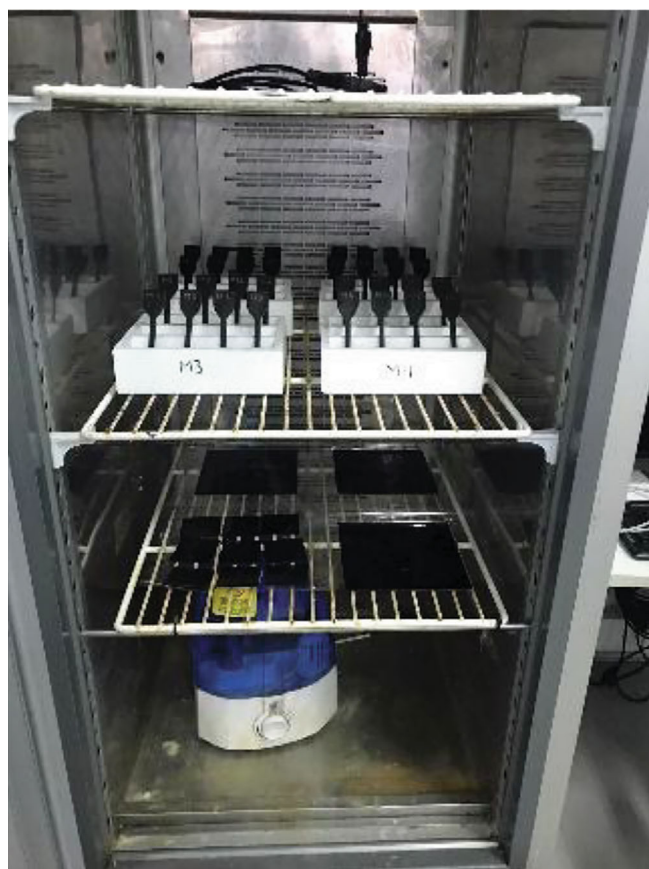
FIGURE 7 Samples in the environmental chamber during the degradation test.
