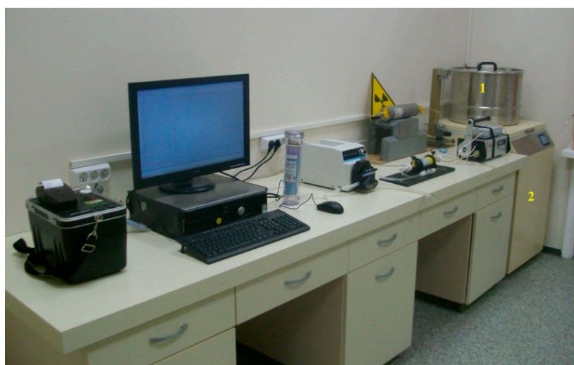
Figure 4. A photo of the exposure facility [9]. The detectors for calibration are placed in the 50 L exposure box (1) that is placed in the programmable thermostat (2).
