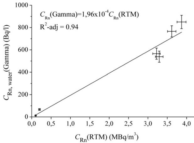
**Fig. 3.** Radon concentration obtained with gamma spectrometry  $C_{Rn,water}(\text{gamma})$  versus obtained with RTM 2100 device  $C_{Rn}(\text{RTM})$ .  $82.5 \times 58$  (1200  $\times$  1200 dpi).
