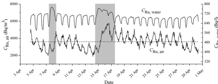
**Fig. 6.** Radon concentration in water and air time series for April, 2012 measured with RTM 2100 and Radon Scout devices respectively. Dashed line indicates monthly average for radon in air which value is 3600 Bq/m<sup>3</sup>. 155 × 72 mm (1200 × 1200 dpi).
