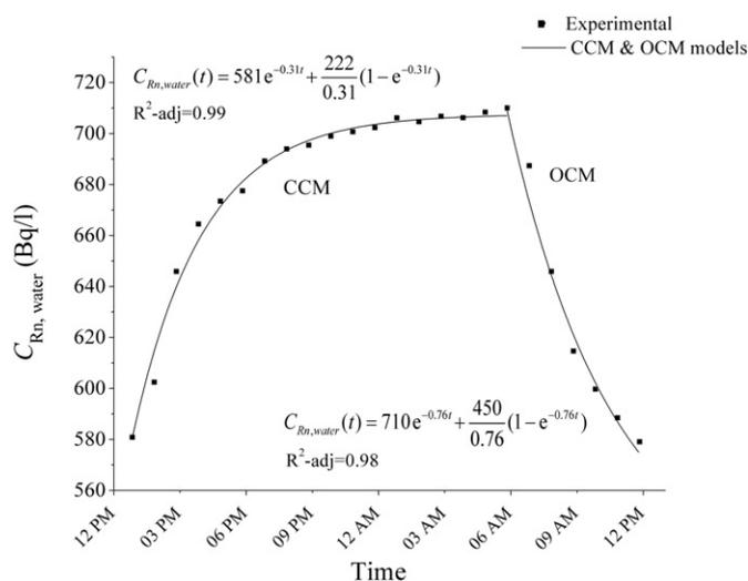
**Fig. 4.** Fit made according to the CCM and OCM models to experimental data on the radon concentration in water from 14th (12:50 PM.) to 15th (11:50 AM.) March. 120 × 90 mm (1200 × 1200 dpi).
