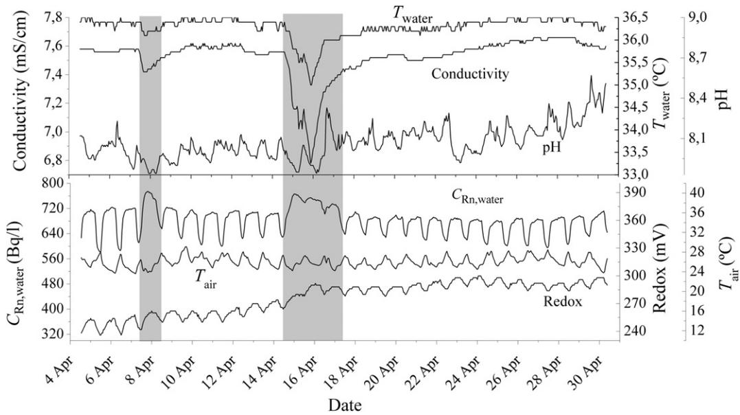
**Fig. 5.** Experimental results of radon concentration in water, conductivity, redox potential, pH and water and air temperatures measured in April with RTM 2100 device. 155 × 85 mm (1200 × 1200 dpi).
