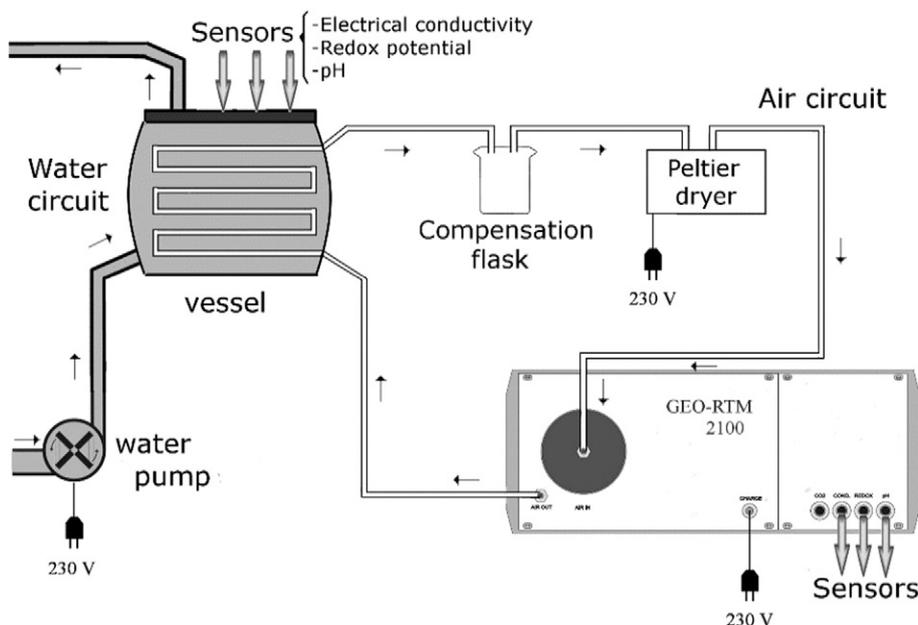
Fig. 2. Experimental device diagram used for continuous measurement of radon in water. 110 × 80 mm (600 × 600 dpi).
