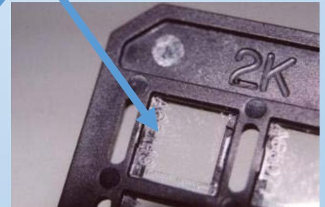
Alpha Particles from Radon and its progeny hit with the detector and leave tracks
