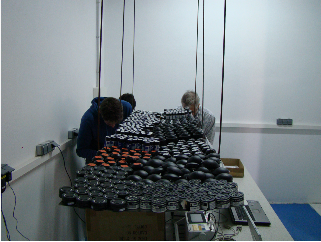
Figure 6: View of position of radon detectors inside the intercomparison room
