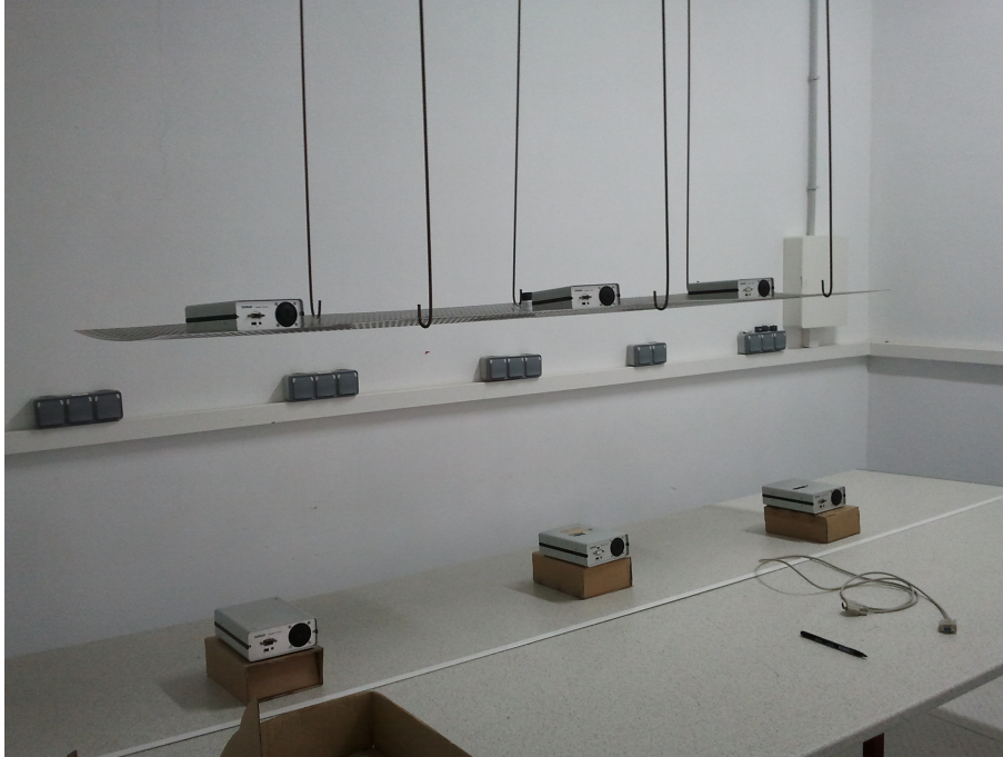
Figure 3: Position of radon Scout monitors used during the inter-laboratory exercise to obtain a reference level of radon exposure
