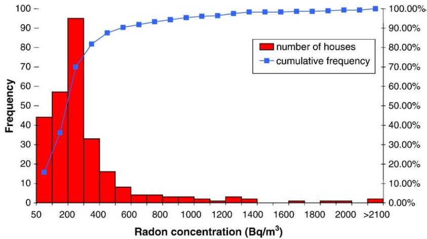
Fig. 1. Distribution of indoor radon concentration in homes in Stei area-Romania.
